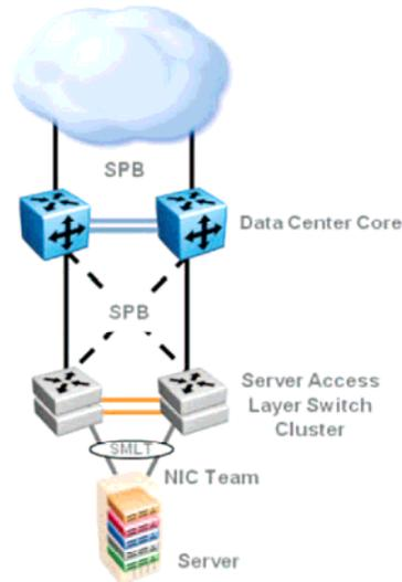
**Figure 2: Fabric Connect Server Connectivity**
