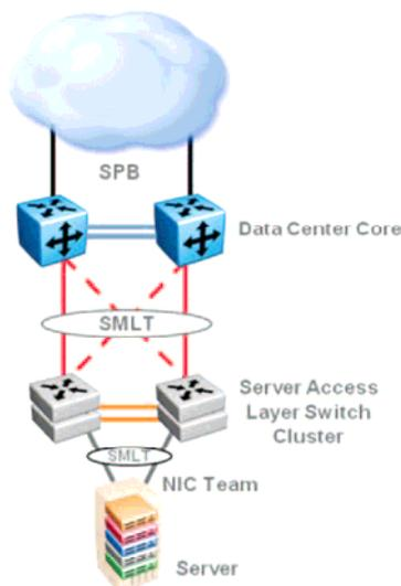
**Figure 3: Traditional Access Switches Connecting to the Fabric Connect Core**
