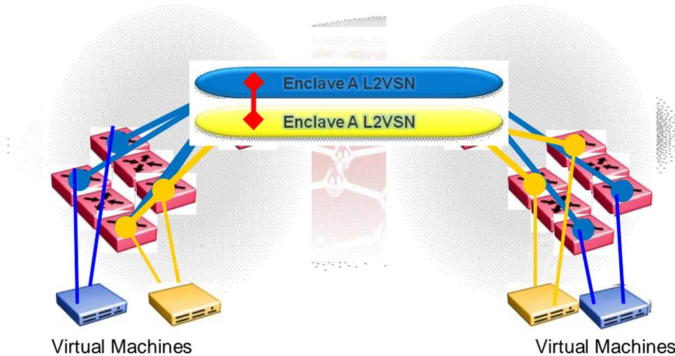
**Figure 6: Inter-Layer 2 VSN Routing**
